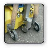
RM-400 has an excellent turning radius by using a differential wheel system.
