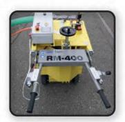
Console leverl engages and disengages the transmission; safety-switch built in
